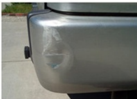
Paint Transfer on a Car
