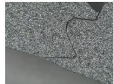
Physical Match of Paint Chip Edges
